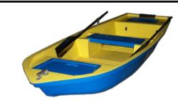
Glass reinforced plastic (fibre glass) is made from fine glass fibres which are combined with a thermoset plastic resin and is moulded. It has a very high strength-to-weight ratio, resists corrosion, water resistant and is light weight. The fibre glass fibres are soaked in liquid plastic, and then pressed or heated until the material fuses together.
